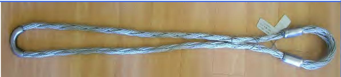
2) *The same strop with knot removed, shows only the faintest trace of set from the knot*
