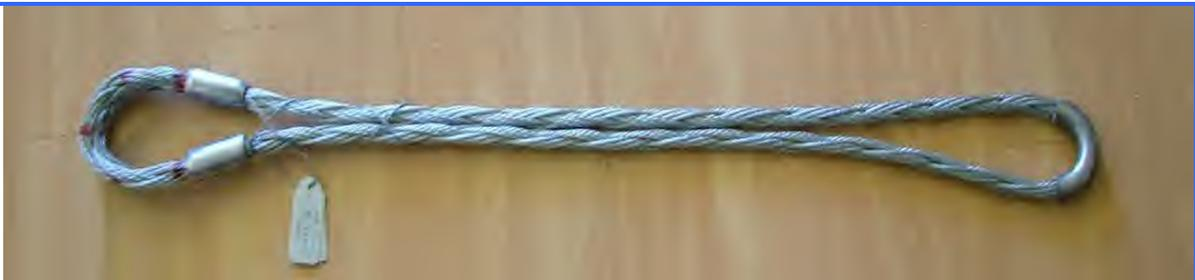
Superflex strop sling in unused condition, size Three/5
