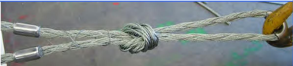
1) *Overhand knot in same strop, load is 300 kg f*
