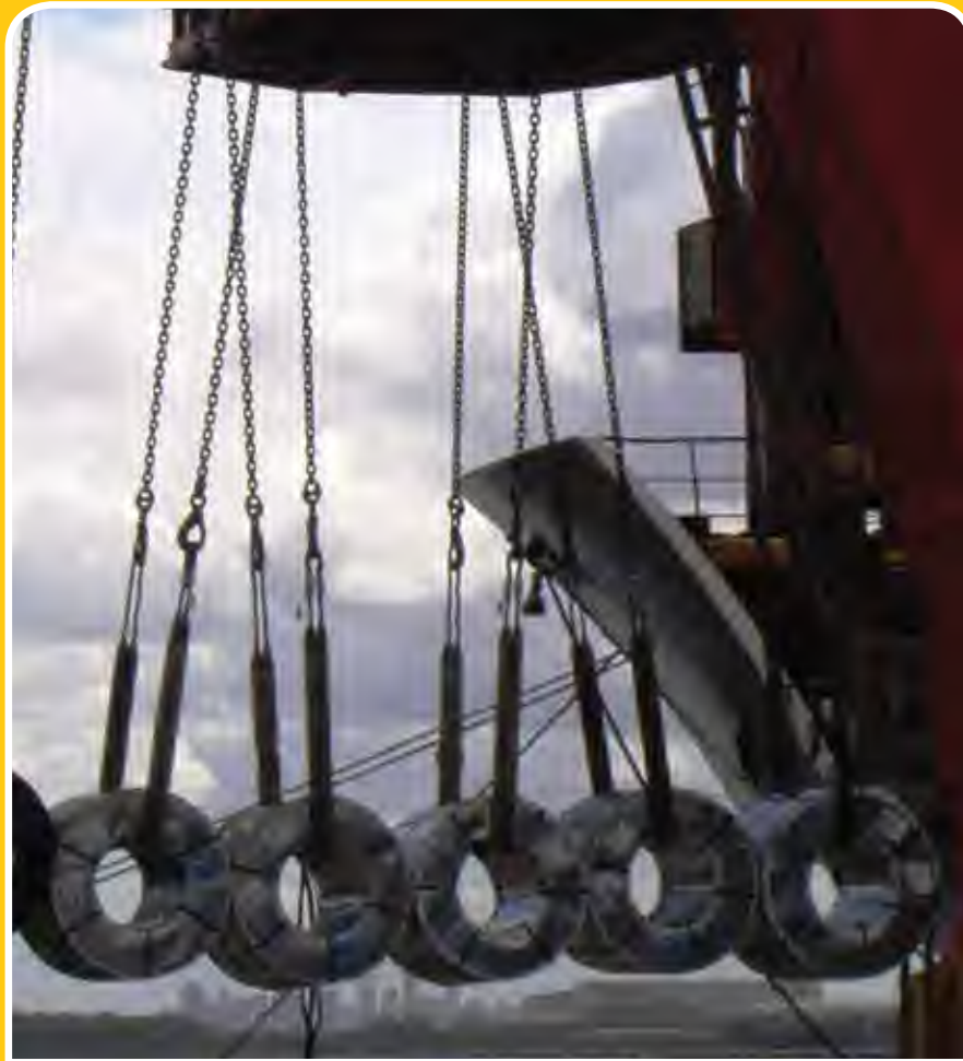
The various designs, based on flat woven steel cable Heavy duty slings for general lifting purposes requiring reduced contact pressure
